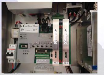
The JTM-30C transmitter consists of one self contained unit ("all-in-one") including Antenna Tuning & Matching circuits and all Transmitter functions all mounted inside an IP66 weatherproof and ruggedized cabinet.
